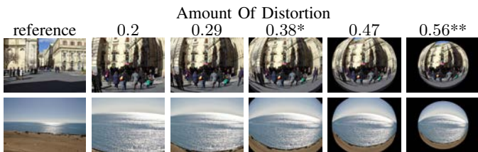
Fig. 3. Two image series from Dataset A. The * and ** symbols denote the full series and full circle distortion rates respectively.
