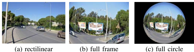
Fig. 1. Examples of perspective (a), full frame (b) and full circle (c) images. The two fisheye images are obtained by artificially adding different amounts of radial distortion to the rectilinear image (a).
