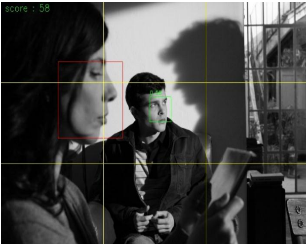
Figure 5. Example of aesthetic assessment for a picture with more than one people. The face on the left has been discarded (thresholds too high): SCORE 58% MOS 42% TOWARDS Not see the face.
