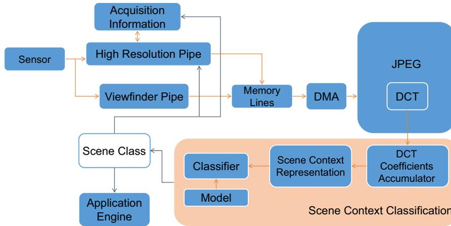
Fig. 7. Architecture of the IGP including the proposed scene context classification engine.
