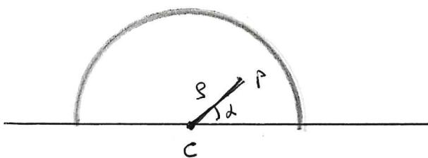
$$\begin{aligned} I_C &= \int s^2 dm = \int s^2 (\sigma s ds dz) = \\ &= \bar{\sigma} \int_0^R s^3 ds \int_0^{\pi} dz = \frac{\bar{\sigma}}{4} R^4 \pi = \frac{R^4}{4} \pi \cdot \frac{2m}{\pi R^2} \\ &= \frac{1}{2} m R^2 \end{aligned}$$
