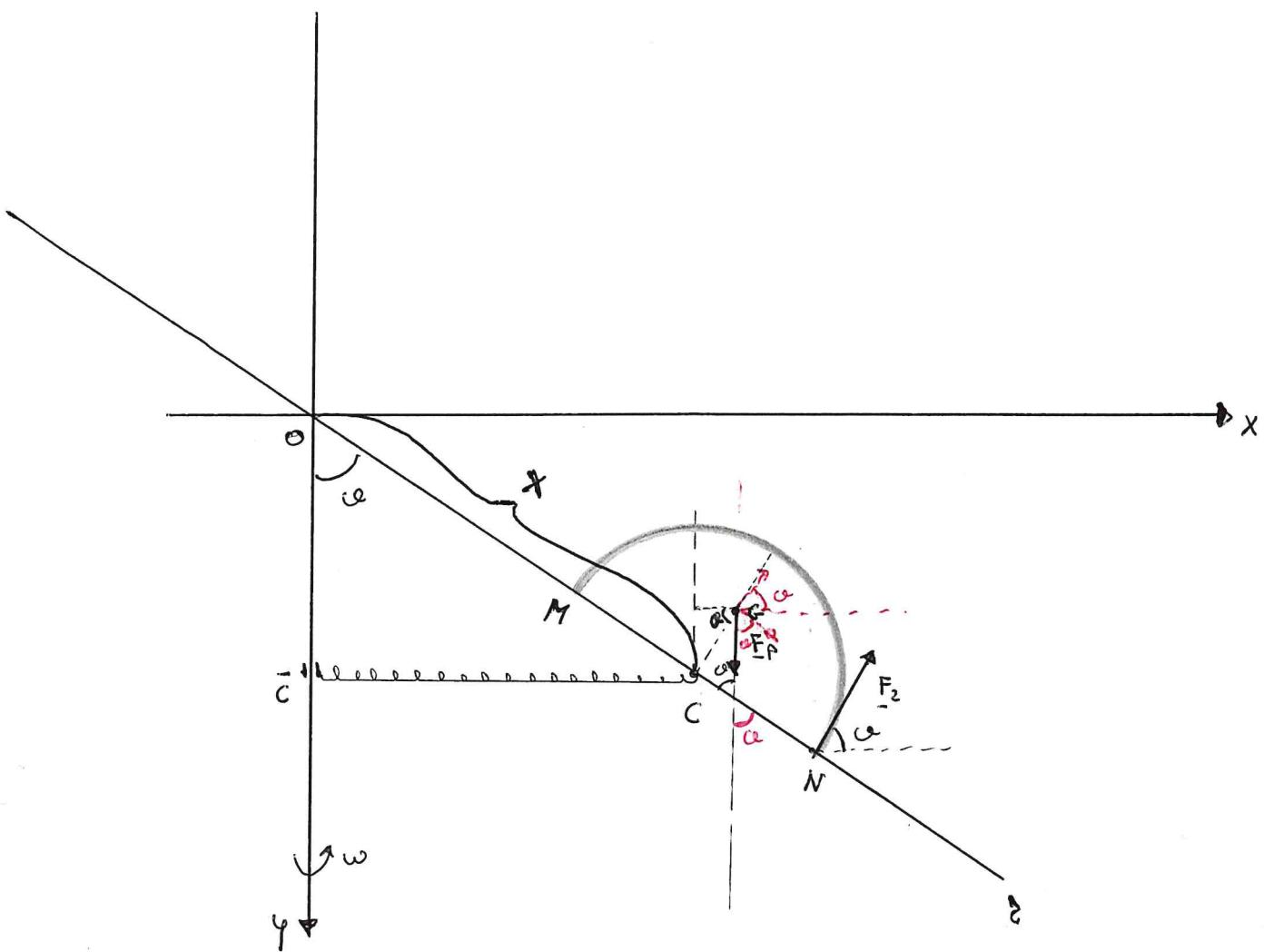
$$C = [x_{\text{senel}}, x_{\text{cosse}}]; \quad M = [(x-R)_{\text{senel}}, (x-R)_{\text{cosse}}]$$
