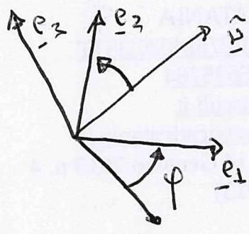
$$\begin{pmatrix} \underline{e}_1 \\ \underline{e}_2 \\ \underline{e}_3 \end{pmatrix} = A_\varphi \begin{pmatrix} \underline{m} \\ \underline{\hat{v}} \\ \underline{e}_3 \end{pmatrix}$$
