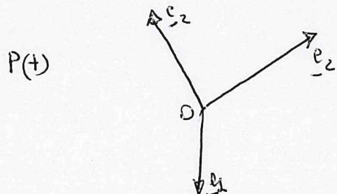
$$P(t) - O' = x_1'(t) \underline{e}_1' \Rightarrow \underline{v}_a = \frac{d \underline{r}}{dt} = \frac{dx_1'}{dt} \underline{e}_1'$$
