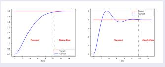
The response of a system to a step (or a pulse is composed of two parts:
