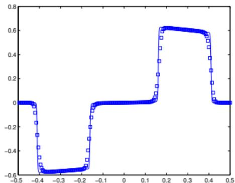
Numerical solutions for the mass density  $\rho$  (left) and the momentum ( $j$ ) (right) in the rarefied regime with  $\varepsilon = 0.7$ ,  $\alpha = 0$  and  $\Delta t = 0.0025$  and  $\Delta x = 0.005$  at  $T = 0.2$ . *Reference solution*, obtained using fine grids with  $\Delta x = 0.001$  (1000 spatial cells)
