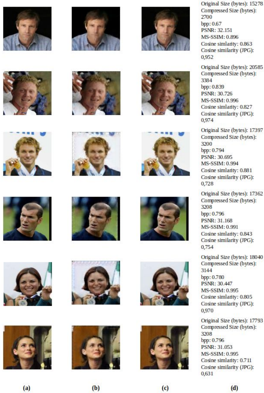
Fig. 3. (a) Original image; (b) Compressed and reconstructed image by our convolutional autoencoder; (c) Image in JPG with quality factor 80; (d) Metrics.
