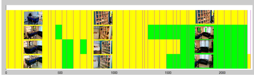
Figure 3: Clustering result applied on four devices. A vertical red line indicates when a clustering block is performed over time, this happens when one of the devices change his subject (e.g. in correspondence of a intraflow change in Figure 2) or at most every 2 seconds.
