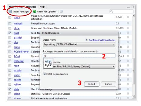
We are going to install the package – rgl (useful to plot 3D images). It does not come with the original R install.
