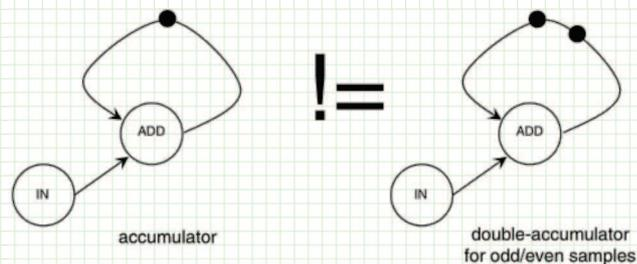
Schaumont, Figure 3.16 - Loops in SDF graphs cannot be pipelined
