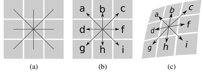
**Fig. 2.** (a) The 4 main directions in a  $3 \times 3$  neighbourhood. (b) The 8 simple directional derivative estimates. (c) An example of distorted (non-Euclidean) neighbourhood.
