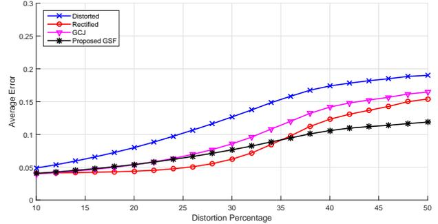
Fig. 6. The mean error for different gradient estimators on the considered dataset at varying of the distortion percentage.
