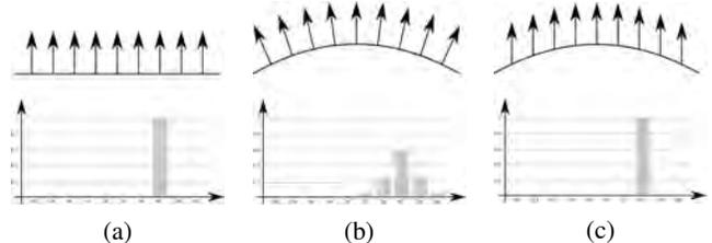
**Fig. 1.** Gradient estimation of a simple feature (i.e., an edge) deceived by distortion. Top row: simple features and the estimated gradient vectors. Bottom row: histograms of gradient orientations. (a) Rectilinear feature. (b) Distorted feature (e.g., acquired with a wide angle sensor). (c) The gradient vectors as they should be computed taking into account the distortion [11].
