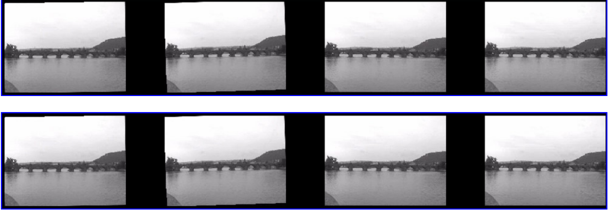
Figure 3. Example of image composition: (top) four destabilized consecutive frames of a real sequence, and (bottom) stabilized sequence.
