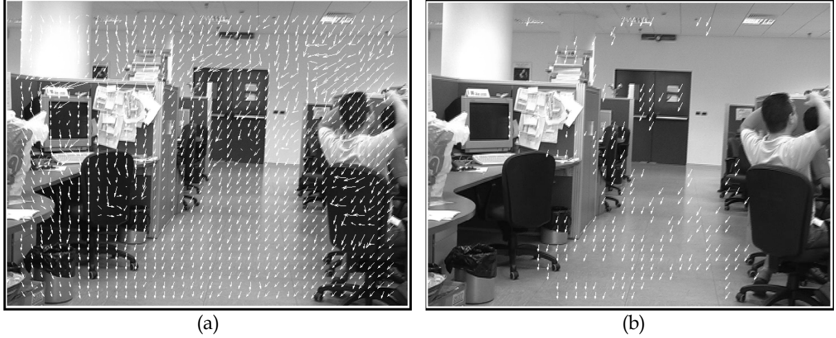
Figure 1. Achieved motion vectors: (a) motion vectors obtained by a block matching algorithm operating in 16 \times 16 blocks, and (b) residual vectors after the filtering process.
