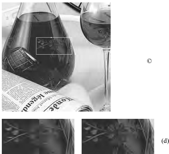
Figure 10: (a) an example of tile classification. (b) Compression obtained by standard Jpeg2000. (c) Compression obtained using the proposed approach. (d) Tiles highlighted in (b) and (c) enlarged to show the different performances.
