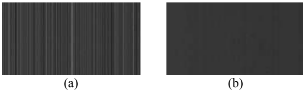
Fig. 2 (a). Visible FPN columns in a frame captured in almost complete darkness. (b) After FPN removal.
