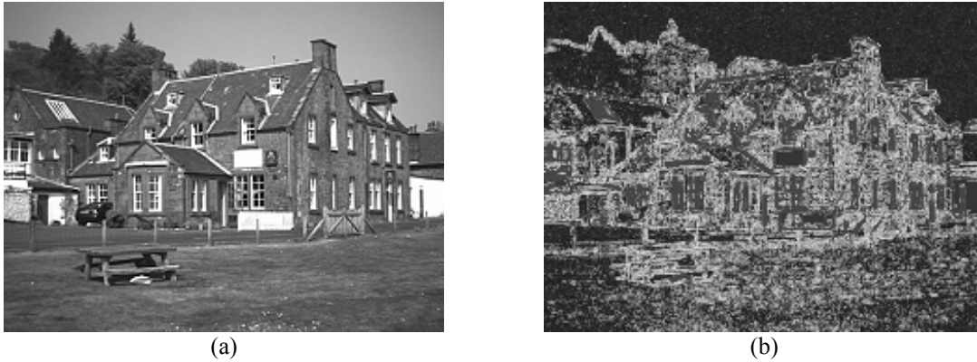
Fig. 5 (a). A CFA video frame. (b) The CFA frame as seen from the texture analyzer: Dark regions are the homogeneous detected areas; bright areas contain different degrees of texture.
