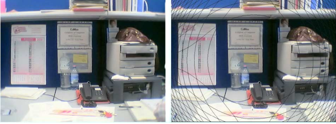
Figure 2 - (a) distorted image; (b) barrel corrected image (some distortion lines are plotted over the image).
