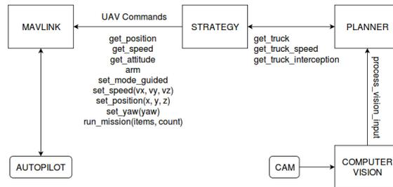
Figure 4. Software architecture.
