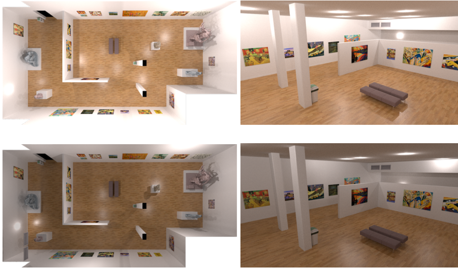
Fig. 2. Two renderings, a plan view and an interior view, of two different optimal light configurations in the art gallery environment.
