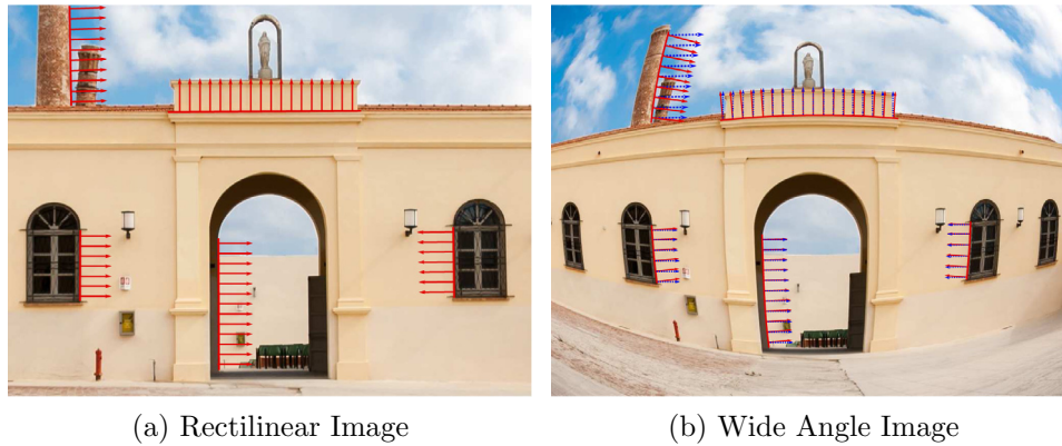
Fig. 1. Gradient estimation of not-distorted and wide angle images. (a) A not-distorted image along with the gradient directions (solid red arrows) of some sample edges. (b) Wide angle counterpart of (a) along with the gradient directions (solid red arrows) of some sample edges deformed by the radial distortion. The ideal gradient directions are reported as dashed blue arrows. (For interpretation of the references to colour in this figure legend, the reader is referred to the web version of this article.)
